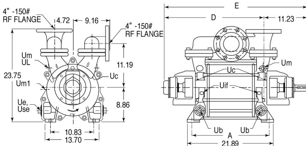
NOTE : Service Liquid is supplied to only one of the  $U_b$  connections.
